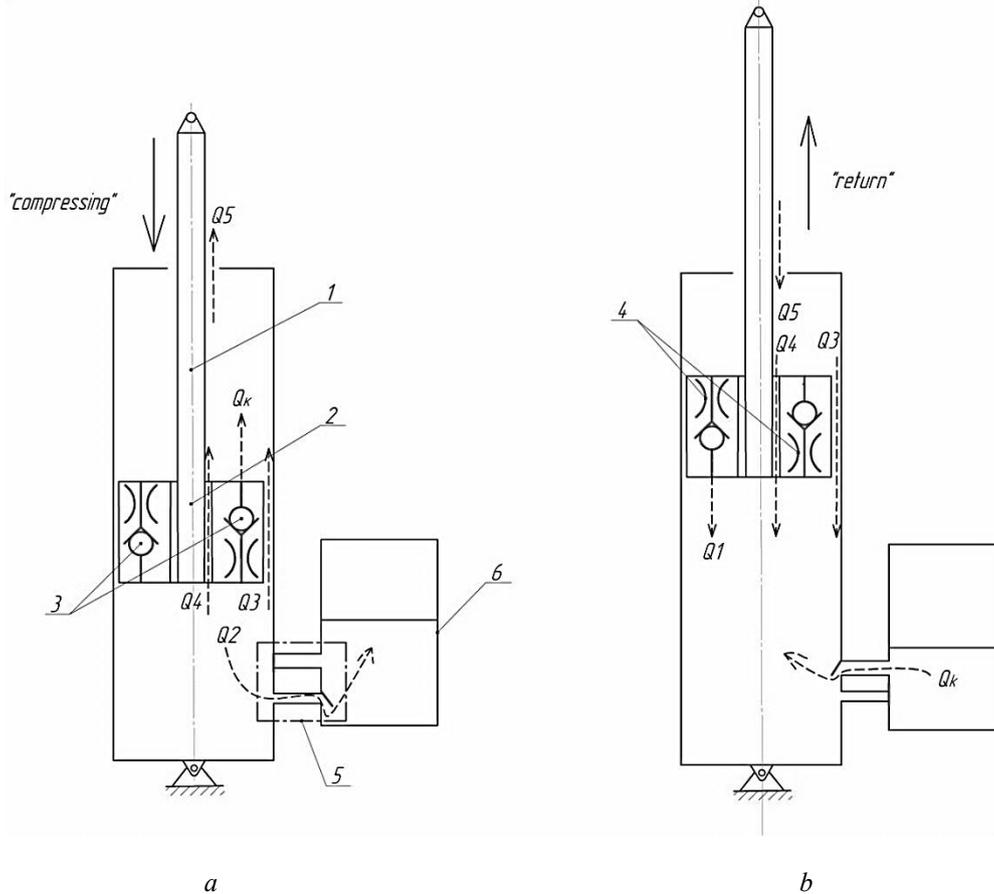
**Fig. 1. Simplified scheme of a hydraulic two-chambered shock absorber: a–flows in the "compressing mode" b - flows in the "return mode"**
