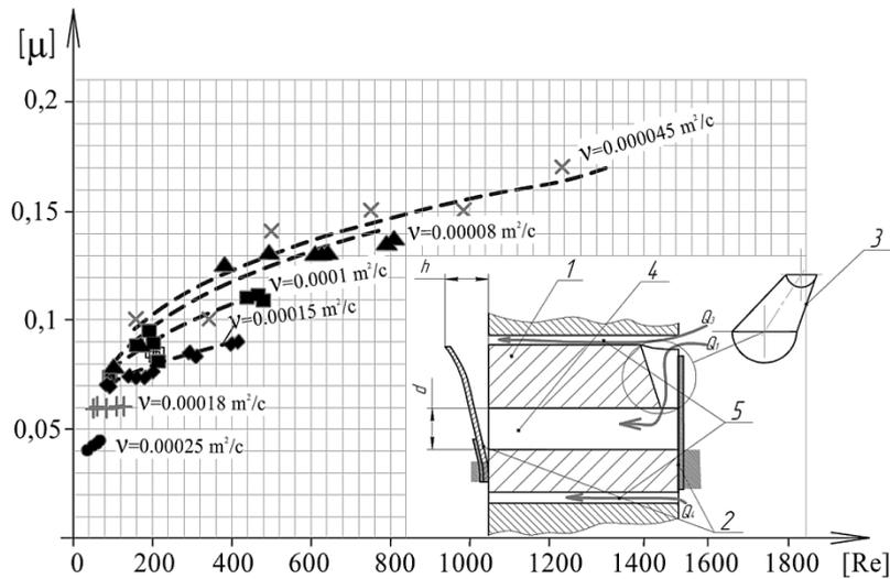
Fig. 5. Dependencies of the working piston flow rate coefficient on Reynolds numbers for the HL-P fluid type
