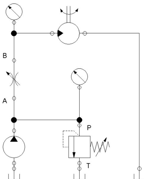
Fig. 1. Hydraulic system with fixed displacement pump and pressure relief valve
