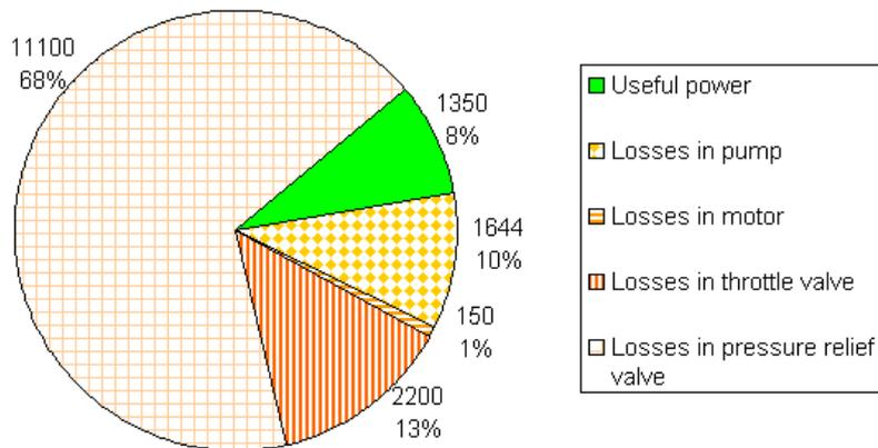
Fig. 11. Energy balance of power in fourth version of operation
