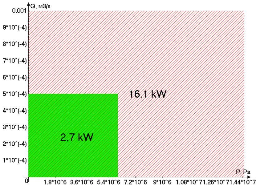
Fig. 8. Useful and supplied power in the third variant:      – useful power;  – supplied power
