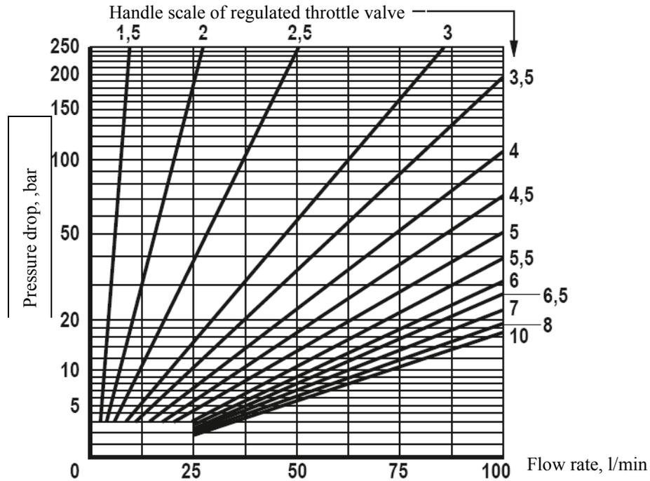
Fig. 2. Characteristic  $\Delta p - q_v$  (Pressure drop – Flow rate) of regulated throttle valve NG16 type
