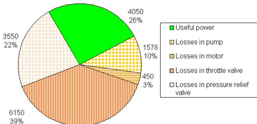
Fig. 7. Energy balance of power in second version of operation
