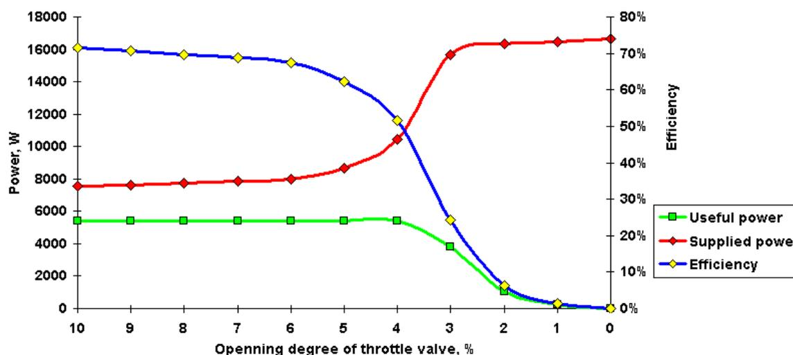
Fig. 14. Diagram of energy balance by different opening degree of throttle valve
