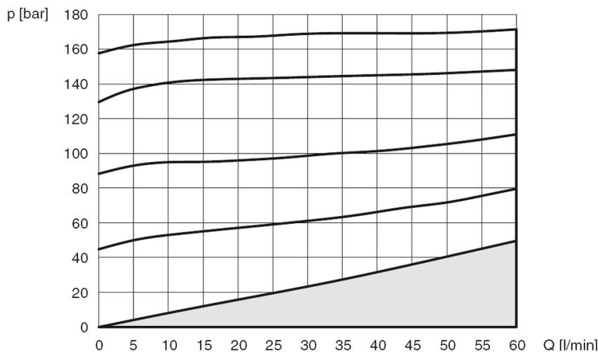
Fig. 5 Characteristic p - qv (Pressure – Flow rate) of pressure relief valve
