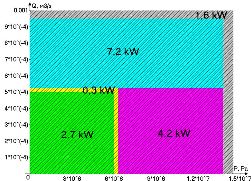
Fig. 13. Supplied and useful power in the third variant of operation: – supplied power (16 kW); – useful power (2,7 kW); – losses in hydraulic motor (0,3 kW); – losses in throttle valve (4,2 kW); – losses in pressure relief valve (7,2 kW); – losses in pump (1,6 kW)
