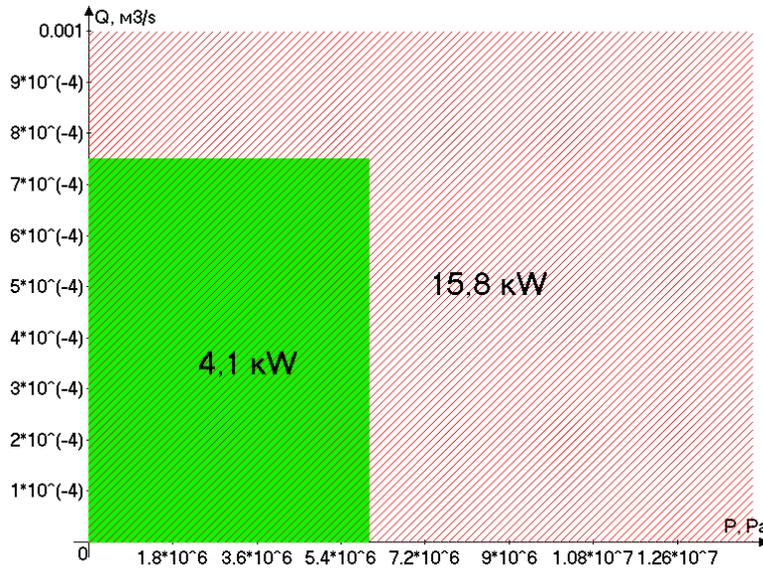
Fig. 6. Useful and supplied power in the second variant: – useful power; – supplied power
