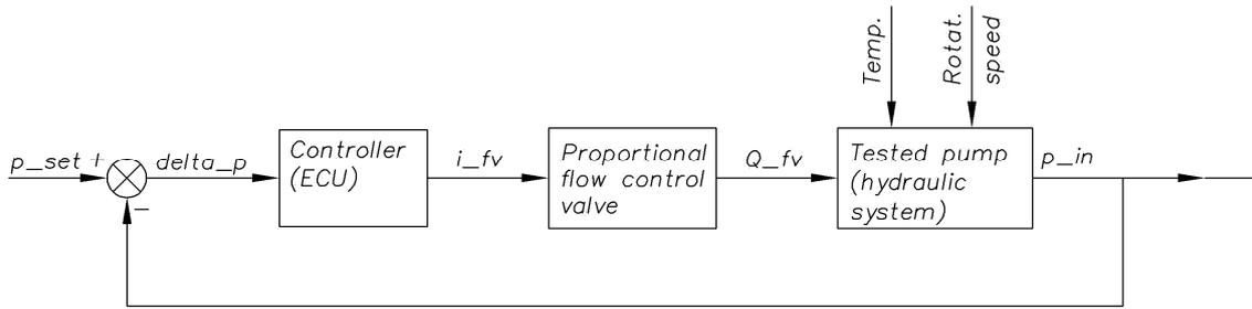
Fig. 3. Control system of the input pressure in the tested pump
