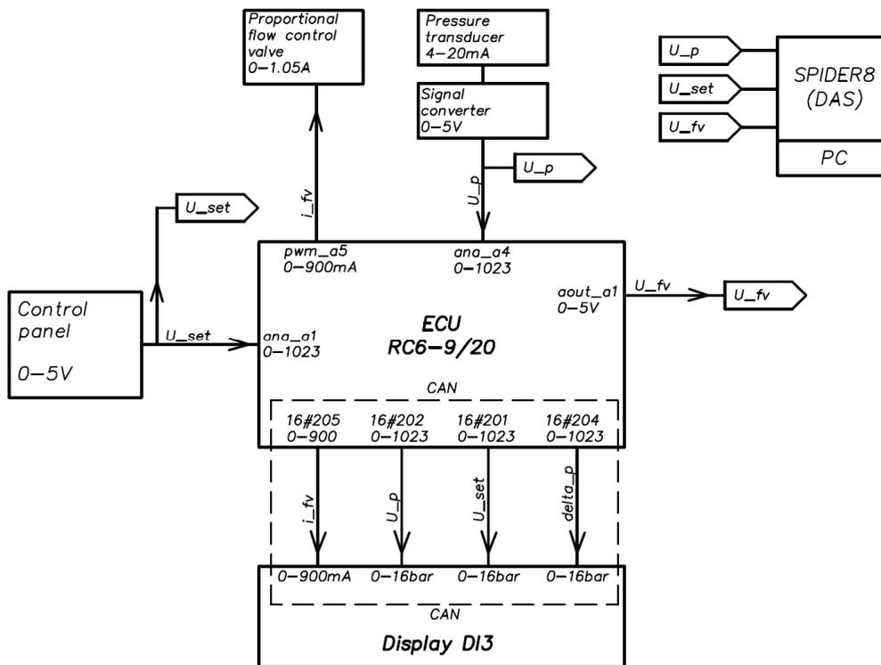
Fig. 4. Flow diagram of signals in the control system
