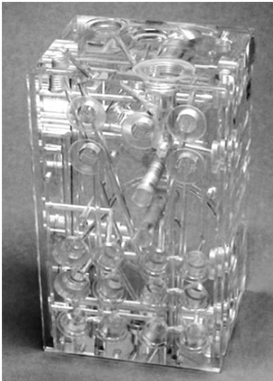
Fig. 1. Example-workpiece with intersection boreholes, Co. HELLER
