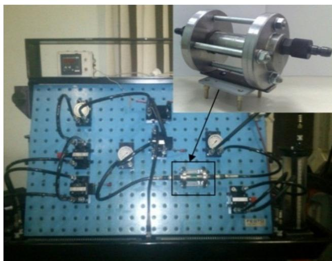
**Fig. 3. Experimental stand for studding “throttle-valve” groups of hydraulic shock absorber (general view)**
