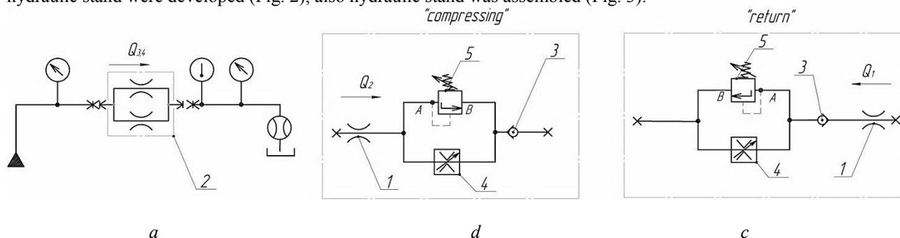
**Fig. 2. Hydraulic circuit diagram of the experimental stand: a- diagram of studding additional throttles flow rates; b- diagram of studding the base valve flow rate; c- diagram of studding the piston throttles flow rate (1-local supplying channel resistances, 3- check valve; 4- hydraulic calibrated bores, 5- pressure check valve)**
