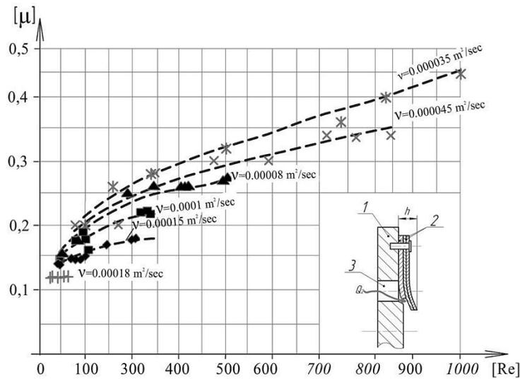
Fig. 4. Dependencies of the base valve flow rate coefficient on Reynolds numbers for the HL-P fluid type
