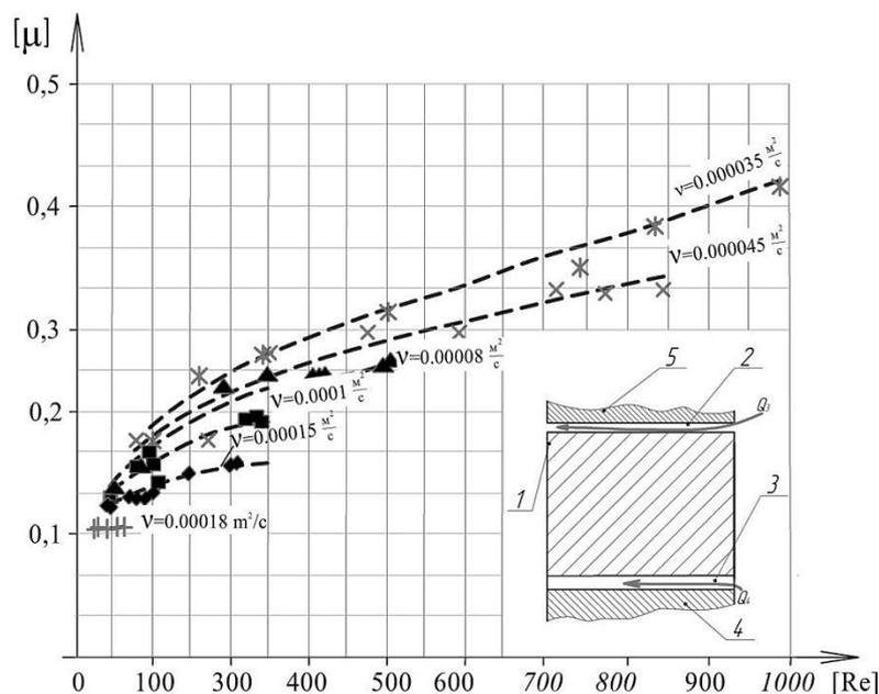
Fig. 6. Dependencies of the additional throttles total flow rate coefficient on Reynolds numbers for the HL-P fluid type
