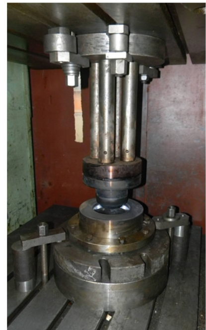
Fig. 8. Construction of stamp (a) and photo of stamp on a hydraulic press DB2436 (b)
