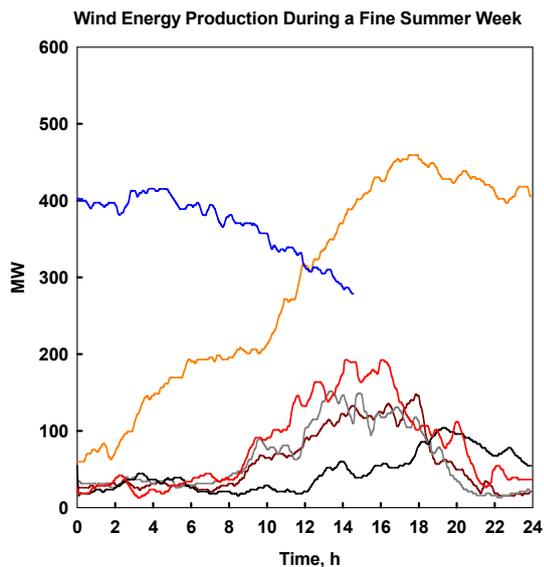
Fig. 3. Power generated by 650-MWel wind turbines in the Western Part of Denmark (based on data from [wdww.wiki.windpower.org](http://wdww.wiki.windpower.org)). Shown summer week (6 days, i.e., various color lines) of wind-power generation
