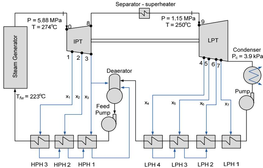
Fig. 12. Thermodynamic layout of 1000-MW<sub>el</sub> VVER-1000 PWR NPP (Dragunov et al., 2015)
