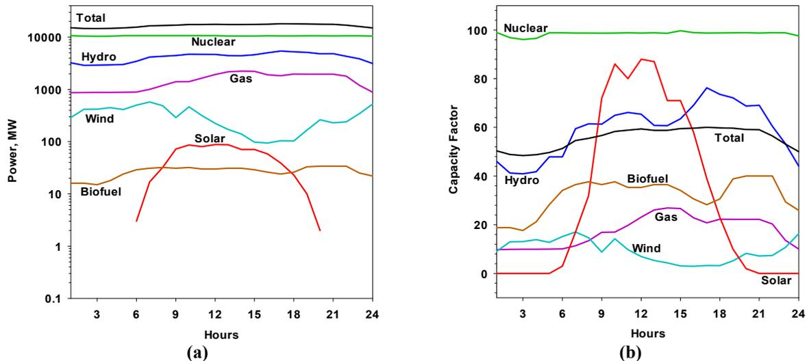
Fig. 10. Power generated (a) and capacity factors (b) of various energy sources in Ontario (Canada) on June 17, 2015 (based on data from <http://ieso.ca/imoweb/marketdata/genEnergy.asp>) (shown here just for reference purposes)
