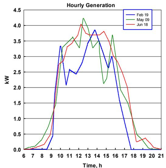
Fig. 4. Power generated by photovoltaic system in New York State (USA) (based on data from [www.burningcutlery.com/solar](http://www.burningcutlery.com/solar)): Shown three mostly sunny days: February 19th; May 9th and June 18th
