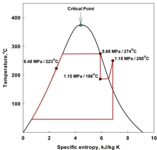
Fig. 13. T-s diagram for a VVER-1000 turbine cycle
