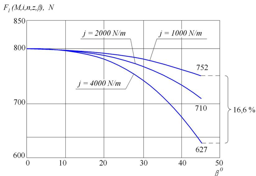
Fig. 5. Compensation of pedipulator driving force drop in the first phase of movement by an increase of the transmission ratio of the servomotor to value  $i=1,2$
