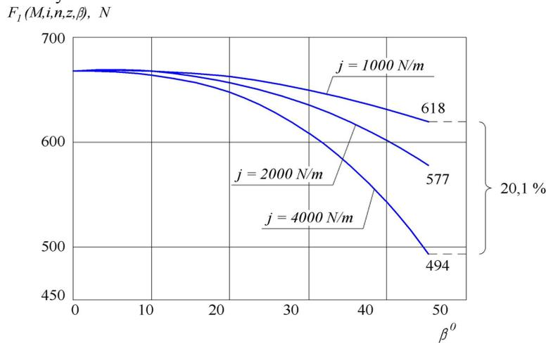
**Fig. 3. Change of pedipulator driving force in the first phase of movement  $\beta = 0 \dots 45^\circ$  depending on the stiffness of the elastic element for the values of the constants: servomotor torque  $M = 10$  N / m ; transmission ratio  $i=1$  ;  $n$  – module of the gearing unit  $n=0,001$  m and  $z$  – number of cogs of the wheel(gear) and the number of its teeth  $z=30$**
