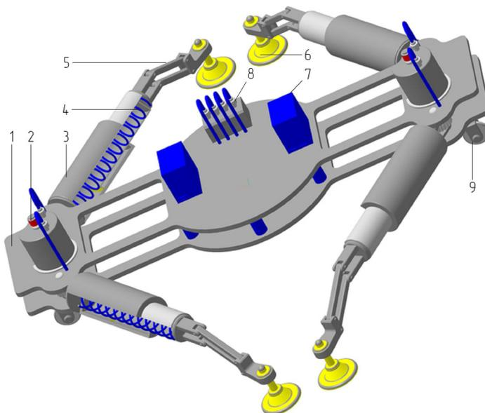
Fig. 1. Climbing robot with energy accumulation and recycling modules
