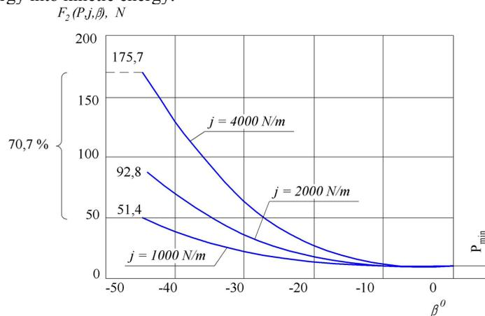
**Fig. 4. Change of pedipulator driving force on the second stage of movement  $\beta = -45^\circ \dots 0$  depending on the stiffness of the elastic elements using same values of the constants (see Fig. 3) and initial compression of the elastic element  $P = P_{min} = 10$  N**
