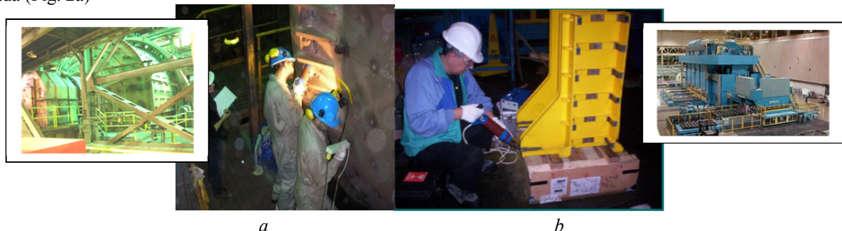
Fig. 2. Application of UP for rehabilitation of welded elements of a) a large grinding mill (left insert) and b) an automotive stamping press (right insert)
