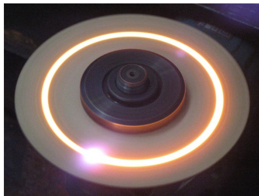
Fig. 6. Disk treatment during its rotation with the frequency 11000 rpm
