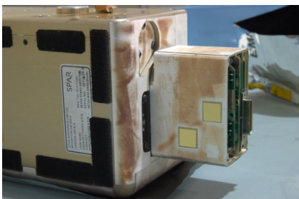
Fig. 6. Visual appearance of the camera CLPA S/N 206 (TVC S/N 209) (stored in a clean room at MDA) after an eight months storage
