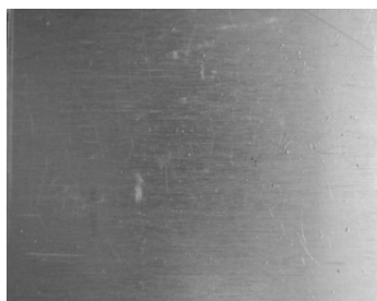
Fig. 7. Appearance of the surfaces of the base metal (a, c) of aluminum alloy of Al-Mg -Si-Cu doping system samples and its welded junctions (b, d) before (a, b) and after (c, d) accelerated tests for resistance against exfoliation corrosion
