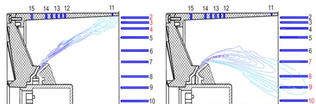
**Fig. 4.** Supersonic jet location determined from pressure probe readings: red probe numbers correspond to greater values of dynamic pressure
