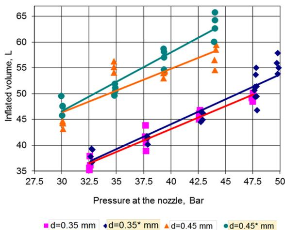
**Fig. 12.** Inflated air volume depending on pressure at the nozzle 0.35 mm and 0.45 mm wide for cases of the base and optimized (marked yellow) design
