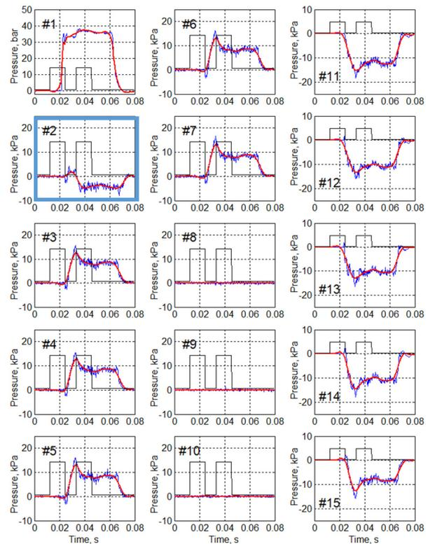
Fig. 9. Pressure patterns in the base inflator model #5.1: slit nozzle width,  $c = 0.35$  mm, motive high pressure,  $P_m = 37.25$  bar
