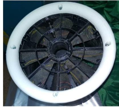
**Fig. 6.** Flow smoothing detail in a form of a rounded leading edge mounted at the inflator inlet
