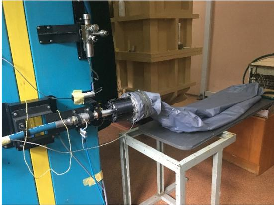
**Fig. 11.** “Big bag” experiments to determine the inflated air volume and aspiration ratio values: measuring 120–160 L bag connected to the aspirated inflator and gas meter
