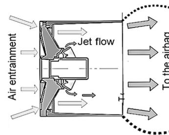
**Fig. 1.** Ejector base design #5.1 and its operation sketch
