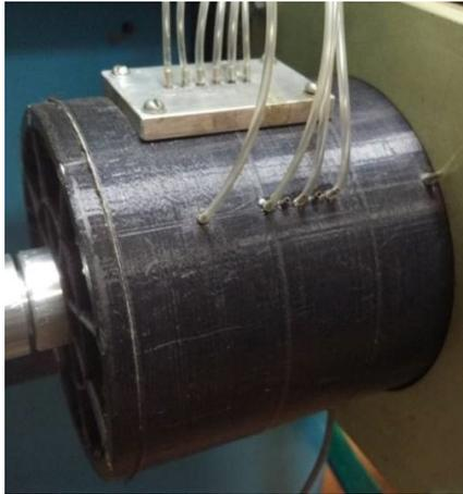
Fig. 8. BPPT installation on the inflator
