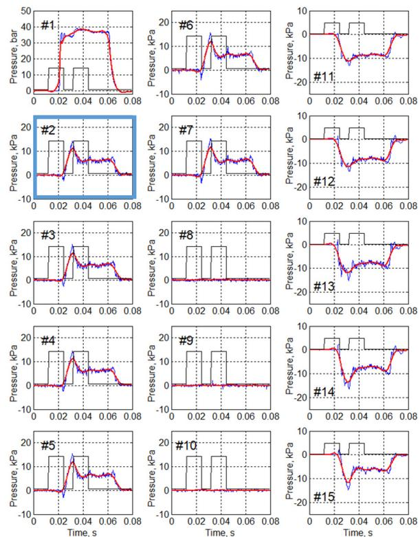
Fig. 10. Pressure patterns in the #5.1 inflator model with the modified inlet: slit nozzle width,  $c = 0.35$  mm, motive high pressure,  $P_m = 38.29$  bar
