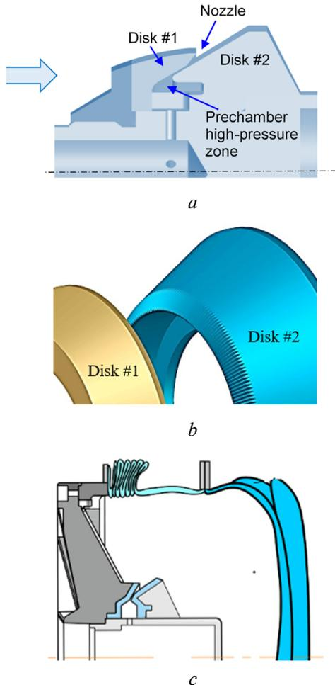
**Fig. 5.** Inflator design modifications tested experimentally: (a) base model with smooth surfaces of the nozzle formed by 2 disks; (b) ribbed jet-forming surface of disk #2; (c) folded mixing chamber
