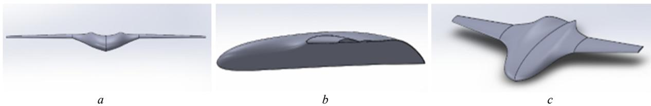
Fig. 2. Proposed Hybrid body design a) Front view b) Side view c) Isometric view
