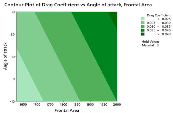
Fig. 9. Influences of Angle of attack and frontal area on the drag coefficient
