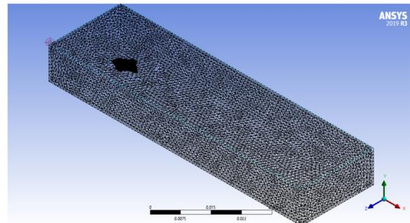
**Fig. 4.** Post meshing with element size 0.0001 m
