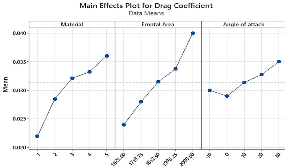
Fig. 6. Main Effects plot showing influences of different parameters on drag coefficient
