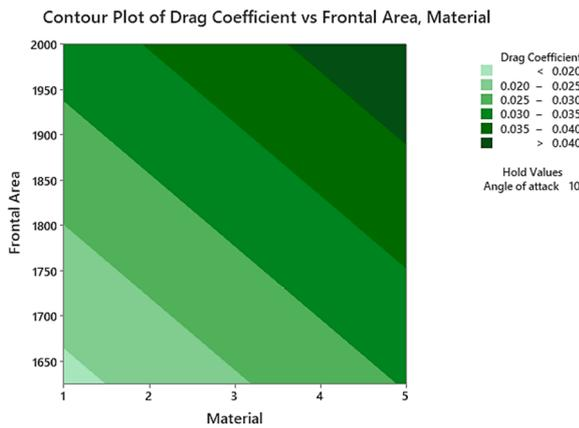
Fig. 7. Influences of Material and Frontal Area on the drag coefficient
