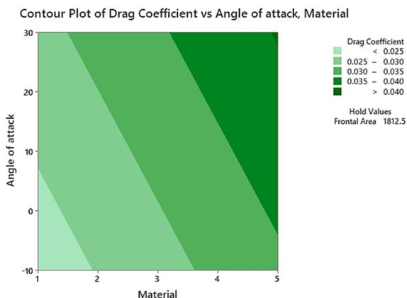
Fig. 8. Influences of angle of attack, material on the drag coefficient
