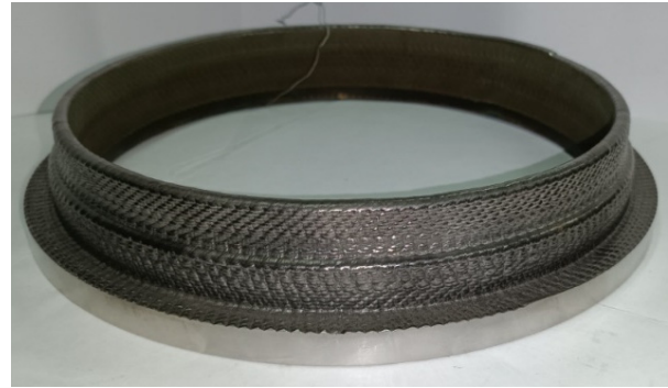
Fig. 12. Appearance of Deposited Workpiece
