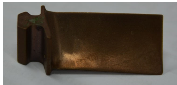
Fig. 5. Avinit Ti-C plasma chemical vacuum-plasma coatings on a mock-up sample of a compressor blade
