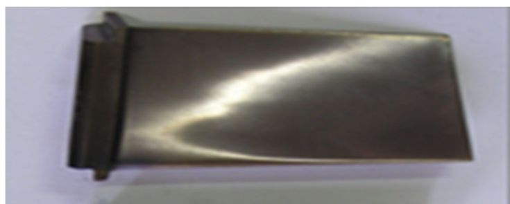
Fig. 7. Plasmochemical vacuum-plasma coatings Avinit Mo-C on a model blade sample. The thickness of the Ti-C coating is 8–8.5 microns. Microhardness 20000 MPa
