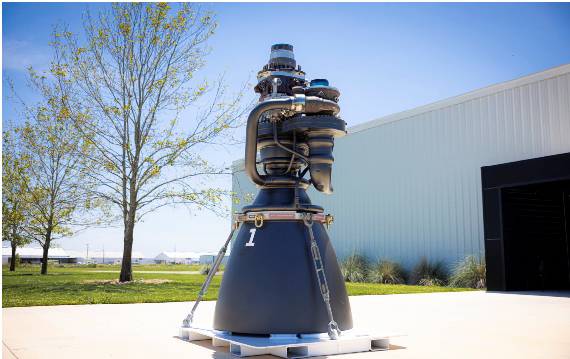
Fig. 1. Engine Raptor 3 manufactured with additive technology by SpaceX
