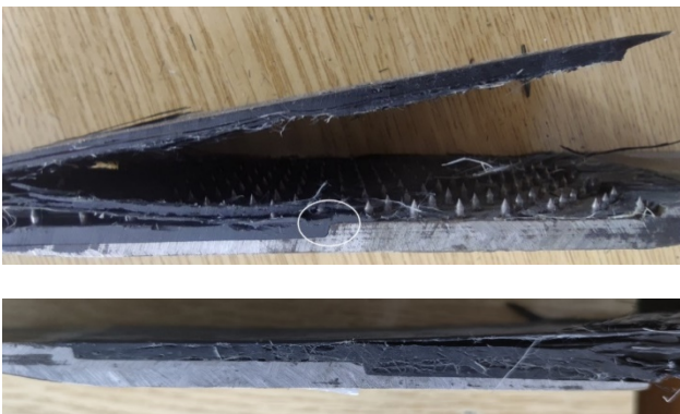
Fig. 11. An example of interlaminar failure mode of composite package at stepped metal article realization (above). White oval shows the location of metal article thickness changing. Side view on the joint is shown below
