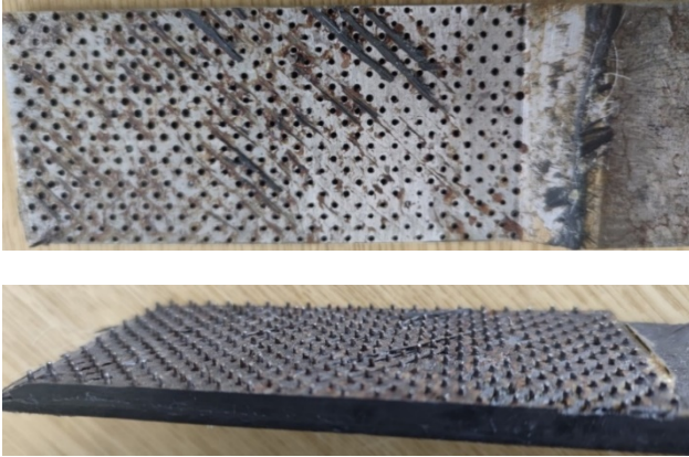
Fig. 10. Appearance of delaminated entire composite package (figure below) from metal tip (figure above). All cylindrical micropins are pulled out fully from metal tip
