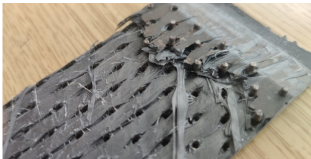
Fig. 14. Top view on delaminated part of composite package
