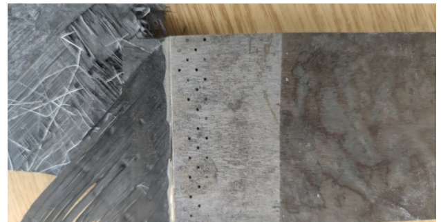
Fig. 13. Typical failure mode of composite package at regular zone neighboring with metal tip. One can catch that several micropins are pulled out fully from metal tip at the rows closest to composite article (black holes)
