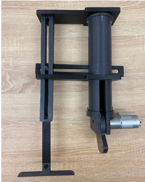
Fig. 12. Experimental prototype of the cam mechanism
