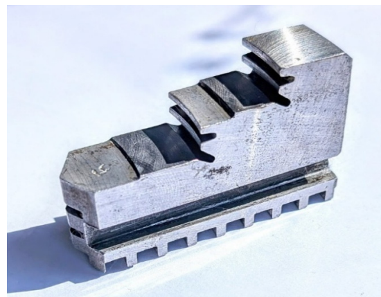
Fig. 2. Steel insert for lathe chuck jaw
