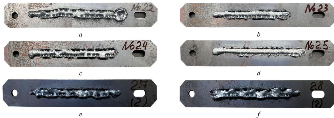
Fig. 4. Appearance of welded weld beads for modes: a – No. 2.2, b – No. 2.3, c – No. 2.4, d – No. 2.5, e – No. 2.7, f – No. 2.8
