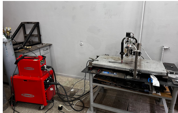
Fig. 1. Automated installation for TIG welding Fronius MagicWave 2200
