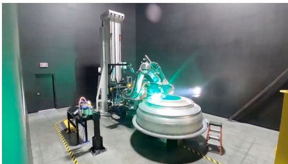
Fig. 2. The process of creating a part of a space rocket using Wire Arc Additive Manufacturing by Relativity Space
