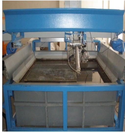
Fig. 1. Schematic diagram of hydro-abrasive cutting setup and waterjet cutting machine
