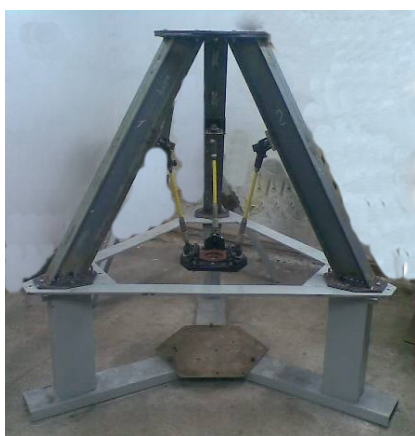
a - frame layout three coordinate drill-mill machine-tool with PKM [7]
