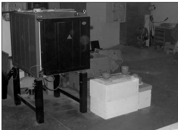
Fig. 5. Electrical Resistance Furnace LAC
