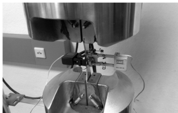
Fig. 3. Axial and cross sectional strain extensometers
