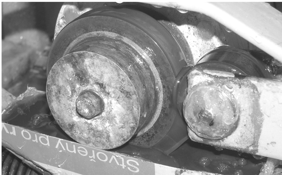
Fig. 2. Relation motion of Workpieces and ceramics wheel (corrosion surrounding with oil)
