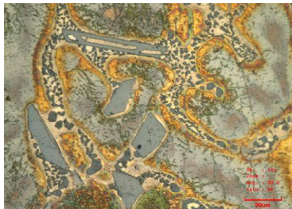
Fig. 7. The microstructure of alloy AlSi8Mg0,3 with addend amount of calcium 1 % Ca (200x magnification)
