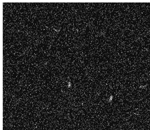
Fig. 15. Scanning EDX analysis of AlZn5,5Mg2,5Cu1,5 alloy after annealing with the temperature of T = 470^{\circ}\text{C} during 8 hours – distribution Cu
