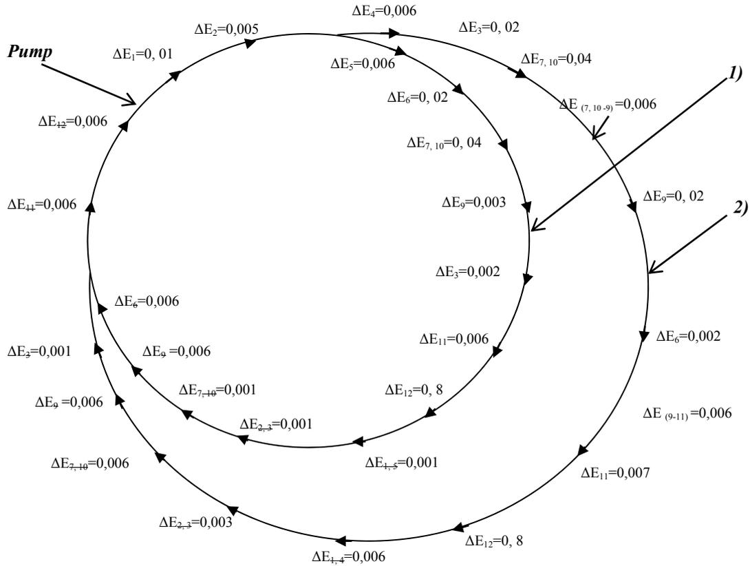
Fig. 4. The distribution of energy loss of the drive with the VB, which operates in the "PULL OUT" at temperatures -20 °C
