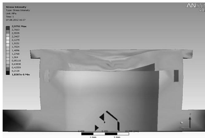
**Fig. 3. Numerical modeling of the valve with flat sealing surfaces deformation under the load**
