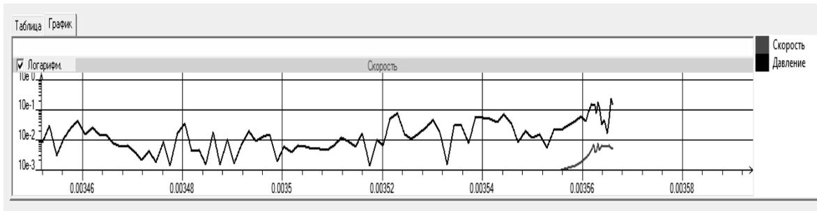
Fig. 5. Graph of velocity and pressure under leakage of jet on the walls of the calibration tube
