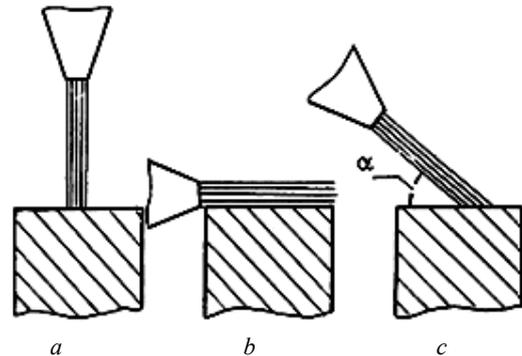
**Fig. 2. Scheme of action of the abrasive jet to the surface**
