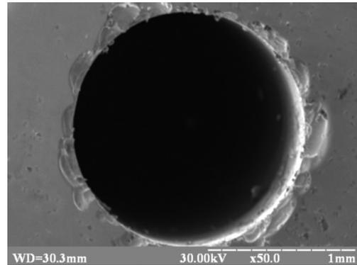
Fig. 4. The photomicrography of the worn edges of the tube
