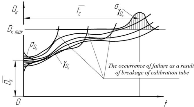
Fig. 6. The dependence of change of the calibration opening on run-in time
