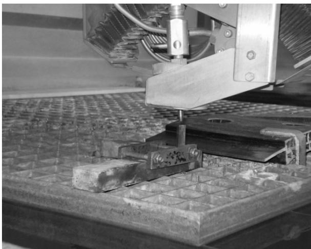
Fig. 8. Installation of a test piece on desktop of hydrocutting machine LSK-5-400
