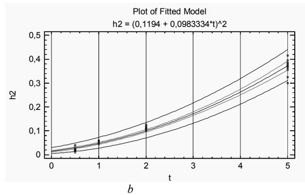
Fig. 9. The comparative diagrams wear of coating TiN (a) and combined coating nitrided + TiN (b)
