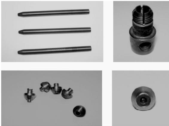
**Fig. 1. Calibration tubes, collet mixing chamber and sapphire nozzle inserts by firm SynergicInc., (Provider – ELFIHmbH. Austria)**
