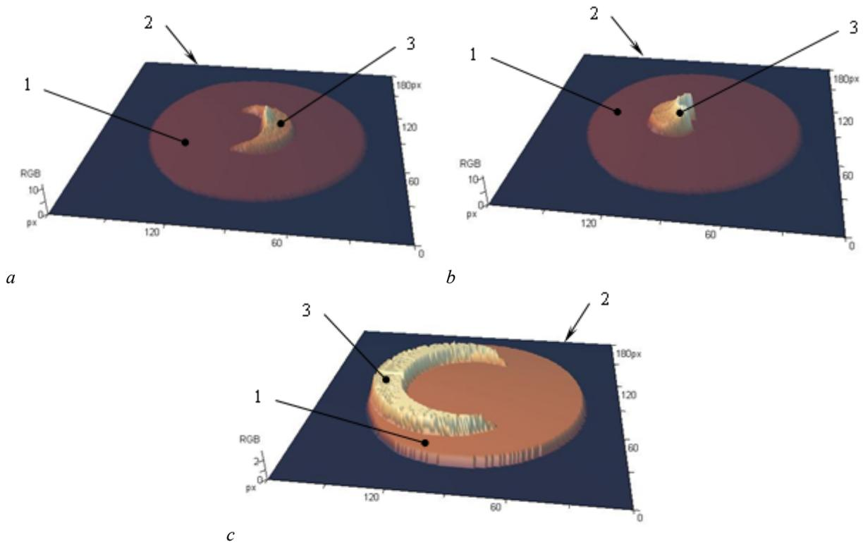
**Fig. 10. Simulation visualization of luminous intensity of the laser beam imprint on the surface of the specimen with misalignment of the jet beam and the refrigerant of 0.18 mm. Orifice hole is made in the shape of a circle**
