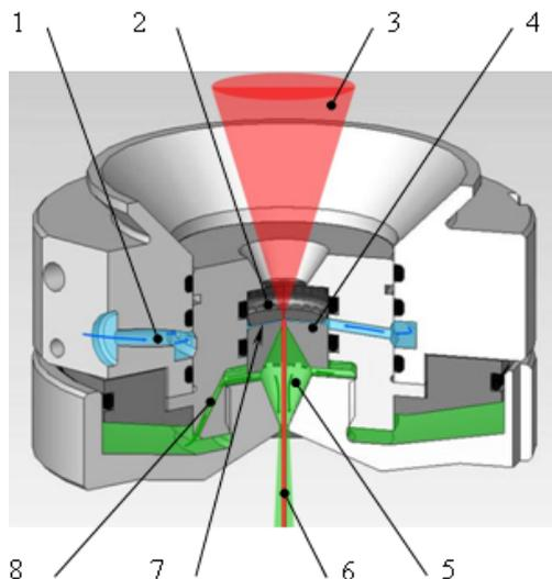
**Fig. 1. An apparatus for forming water jet guided laser stream produced by Synova (Switzerland)**
