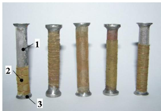
**Fig. 9. Versions of devices for removing of turbulence effect**
