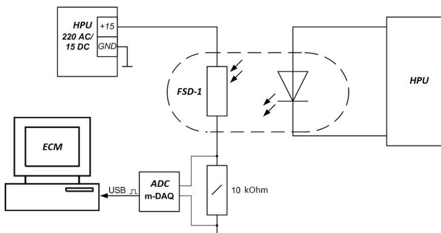
Fig. 7. Schematic diagram of the measuring system based on ADC
