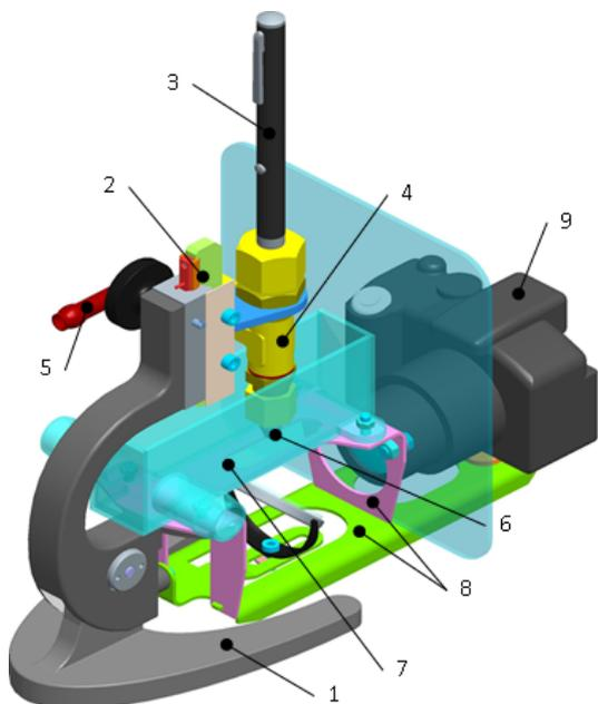
**Fig. 3. 3-D model of the device for coaxial input of beam into a liquid stream**
