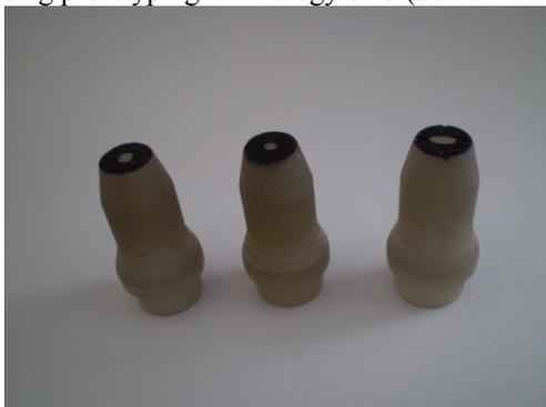
Fig. 5. Nozzles created by prototyping
