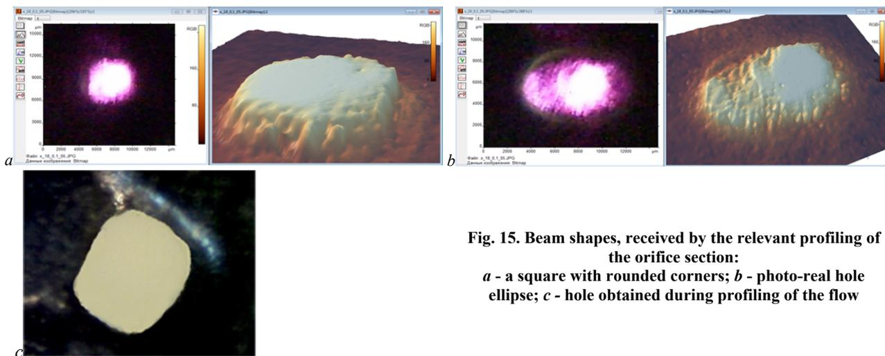
**Fig. 15. Beam shapes, received by the relevant profiling of the orifice section:**
