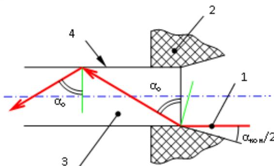
**Fig. 4. Settlement scheme determining the value of a half angle of generatrix of the cone of nozzle transition section**
