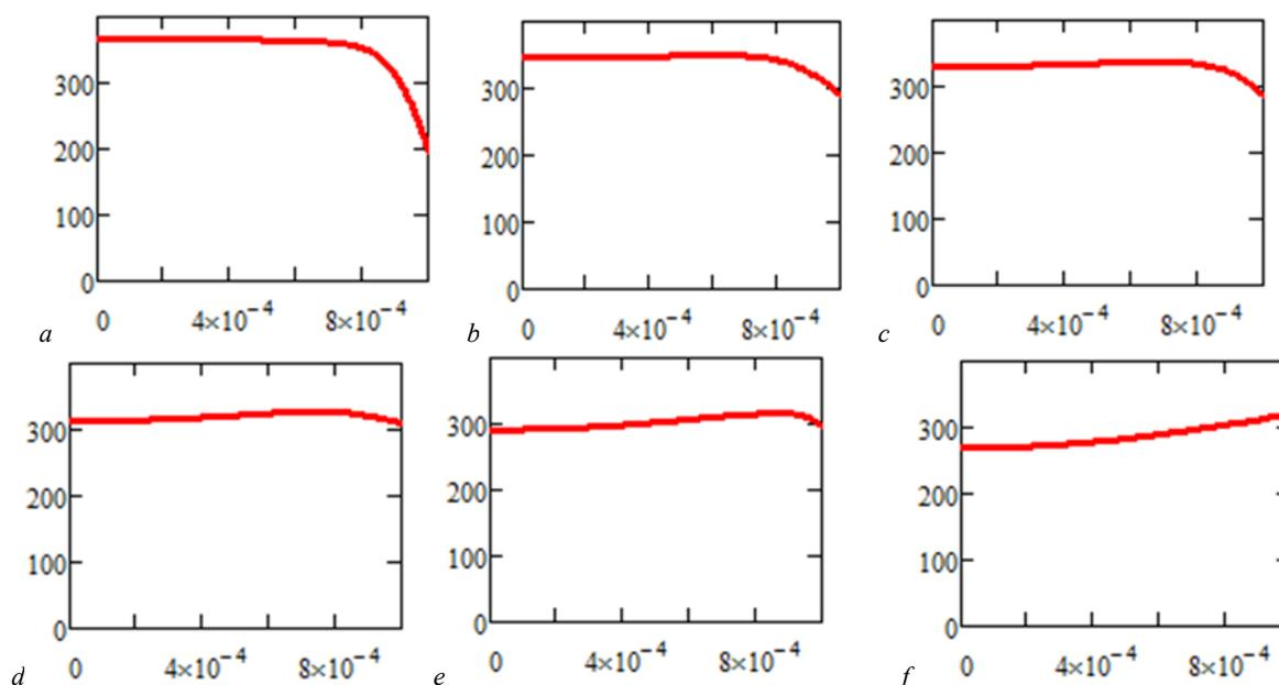
**Fig. 13. Reduction of the flow velocity at the nozzle end face and at each next millimeter of free liquid discharge behind the nozzle, which leads to a corresponding reduction in the intensity of the laser emitting. This graphic representation shows from the jet axis (left) to the boundary of the nozzle hole projection (right):**
