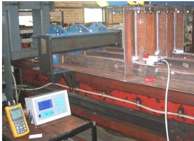
Fig. 10. Measurement of residual stresses using UltraMARS system in large-scale welded panel in as-welded condition and during the fatigue loading of the panel
